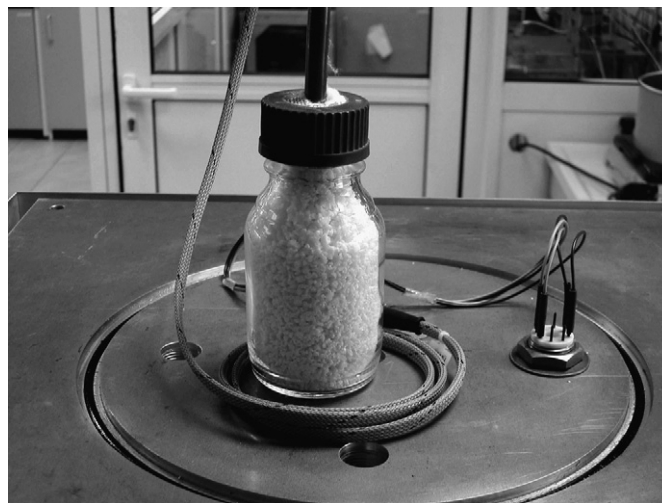
Fig. 9. View of a 600 \text{ cm}^3 bed of granular cellulose acetate aerogel (hot-wire immersed in a divided OA5 bed).
